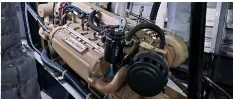
(Above) The 429-kW (575-hp) PowerTech 13.5L engines turn 76x76-centimeter (30x30-inch) props through Twin Disc transmissions with a 2.3:1 gear ratio.
