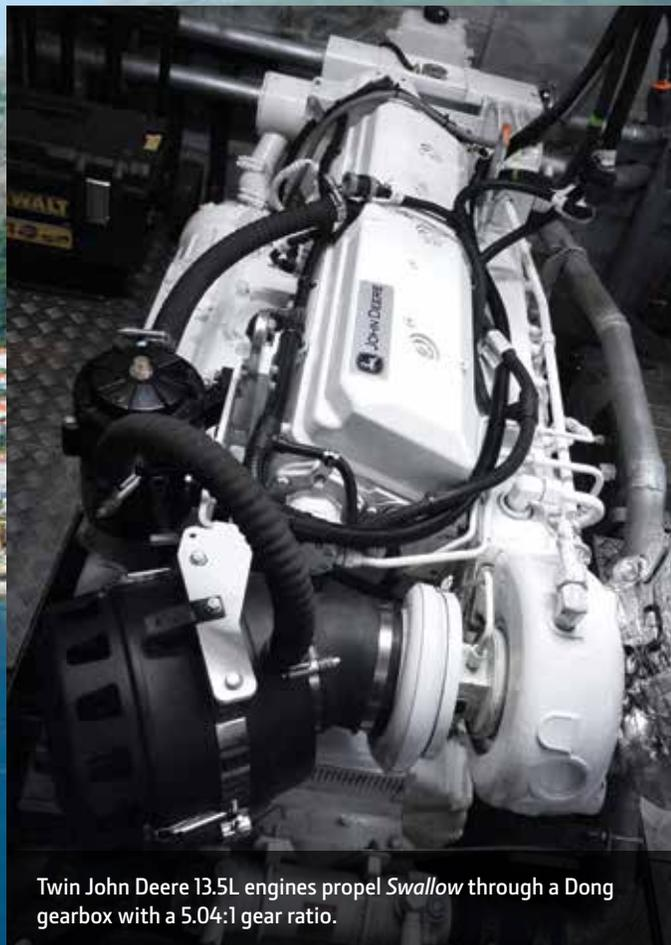
Twin John Deere 13.5L engines propel *Swallow* through a Dong gearbox with a 5.04:1 gear ratio.
