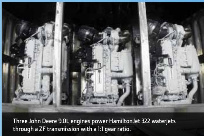
Three John Deere 9.0L engines power HamiltonJet 322 waterjets through a ZF transmission with a 1:1 gear ratio.
