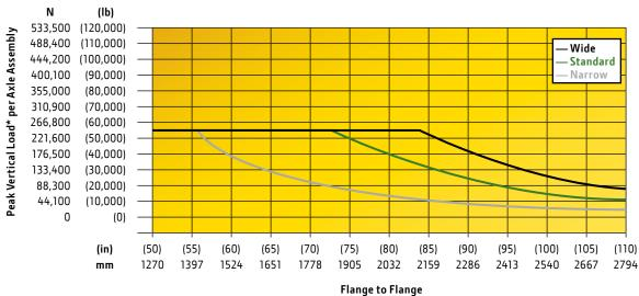
\*Peak load level (fixed axle) assuming traction-limited condition, 0.5 traction coefficient, and a specified loaded tire rolling radius.
