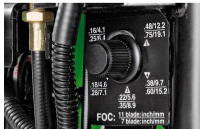
**Adjustable frequency of clip with lockout:** Frequency of clip can be adjusted with a simple dial, then mechanically locked to prevent further changes.
