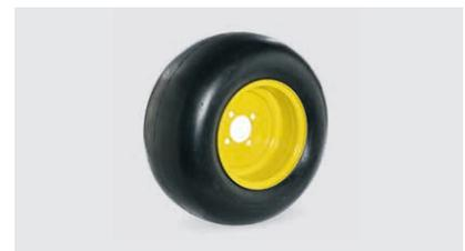
**Balloon tyre (optional):** These rounded balloon tyres tread lightly and reduce sidewall deflection – for an exceptional finish with fewer tyre tracks.
