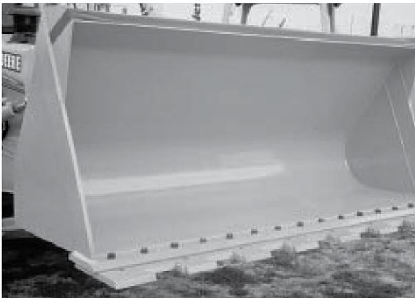
Backhoe loader bucket equipped with T825330 (25.4mm x 152.4mm x 301.63 mm, 5/8-in. bolts) short standard sections, and T825333 and T825334 end sections.
