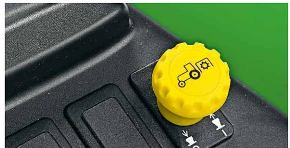
**Independent PTO:** Forget the days of stopping the tractor and manually engaging the PTO. With the electro-hydraulic PTO you can turn on your implement while you're on-the-go, so you can get your work done faster and easier.
