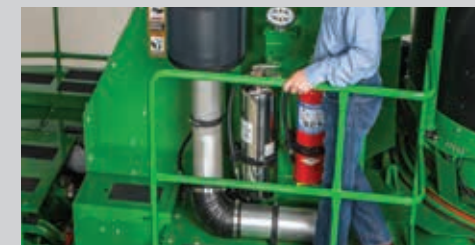
Service platforms have non-skid surfacing and are surrounded by handrails for safe access.
