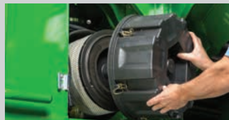
New air filter assembly is better protected and the hood is easier to grip.
