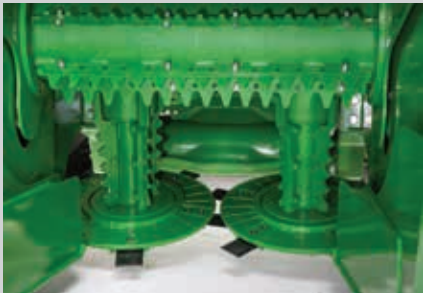
Standard large 61 cm diameter discs or optional 56 cm discs are available.
