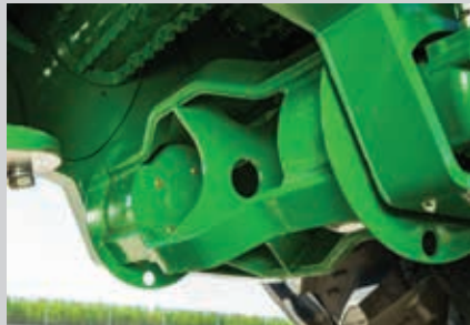
Open buttlifter options minimise soil intake and mud build-up.
