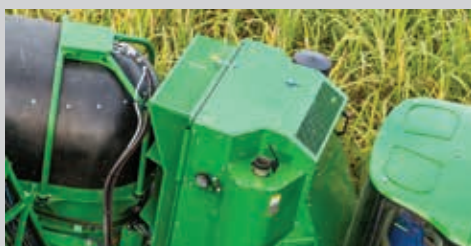
The reversible fan automatically keeps the cooling package clean. With the new variable speed control, it will maintain the engine operating at the appropriate temperature to optimise engine performance.
