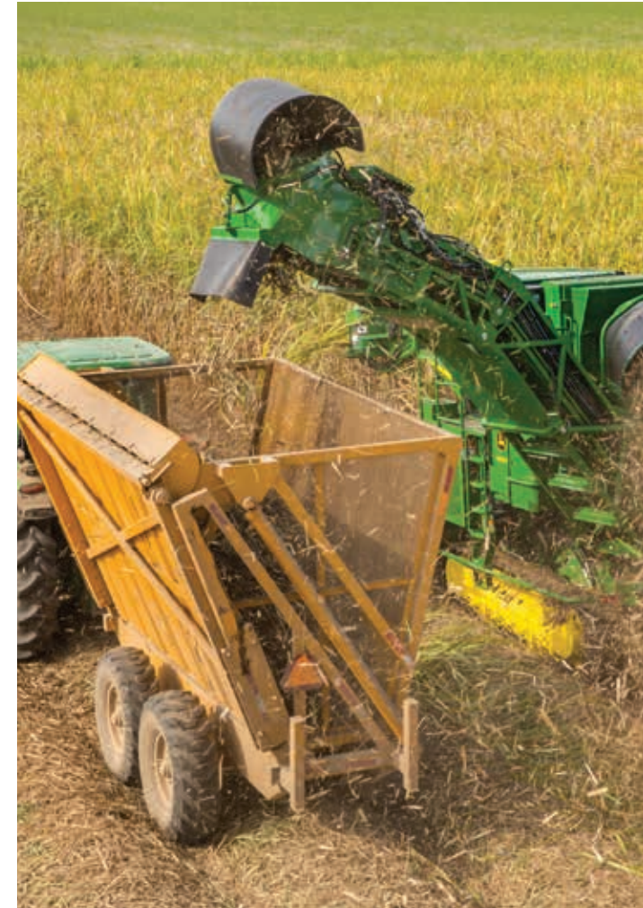
The four-blade, 152 cm diameter fan is the largest in the industry.
