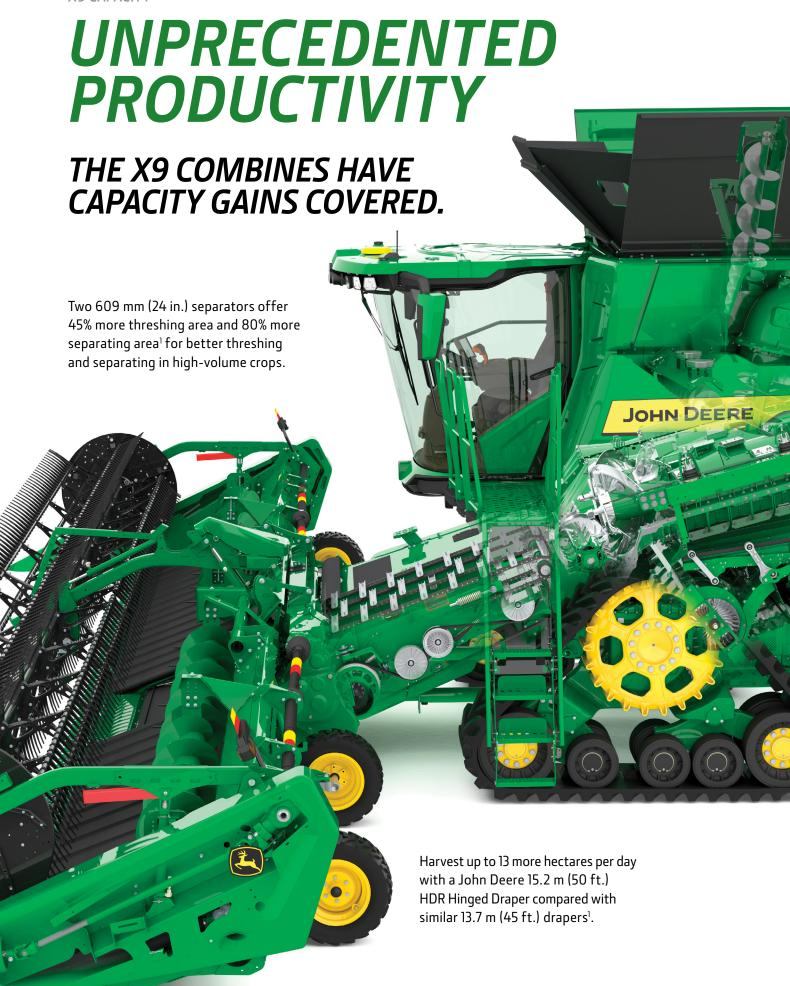
Even with a 23% wider feederhouse<sup>1</sup> and more threshing and separating area, the outside dimensions are about the same as the S790, for tight turns and narrow transport.
