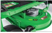
**42in. (107cm) Accel Deep<sup>™</sup> Mower Deck:** Offers no compromises in cut quality and performance when compared to a similar gas machine.
