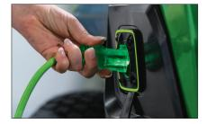
**On-Board Charging:** Just plug in a standard extension cord when you are done mowing and walk away. The Smart Charge Technology prevents over charging and maintains battery life.
