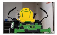
**Intuitive Controls:** Integrated park brake is activated when the control levers are pushed outward. Power button easily turns on machine.
