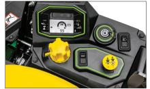
**Operator Display:** Large LCD screen to monitor battery levels and three operator modes to adjust settings that fit operator preference and yard conditions.
