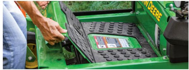
**Adjustable three-position foot platform.** Easily customize its position without tools to find your perfect fit. After mowing, the platform detaches, giving you easy access to the mower deck for cleaning or service.
