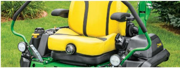
**Adjustable seat.** With unique seats for E, M, R Series, the iconic yellow seat on the Z700 Series now makes mowing more comfortable and with our ComfortGlide™ fore/aft suspension on all M and R Series Z700s.
