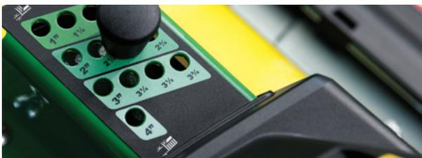
**Cut adjustments in .63 cm (1/4 inch) increments.** For a precise cut, easily adjust from 2.5 – 10.2 cm (1 – 4 inches) on the Z300 Series (vertical pin system) and Z500 Series (as shown above), or 3.8 – 12.7 cm (1.5 – 5 inches) on the Z700 Series (dial adjustment). Pin is magnetic for ease of use on Z500s.
