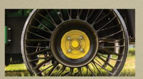
Equip your R model Z700 with the latest in tyre technology with optional MICHELIN® X® TWEEL® Turf airless radial tyres.
