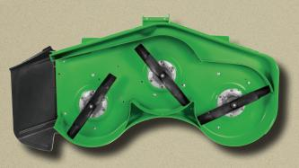
**Z500's High-Capacity Mower Deck.** Forged from our thickest, 9-gauge steel for excellent durability. These 48-, 54- and 60-in. mowers provide a pristine cut thanks to additional deck depth and superior clipping dispersal.
