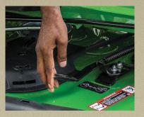
Mulching made easy. The MulchControl<sup>™</sup> Kit lets you mulch with a quick flip of the lever. Grass too tall? Simply flip the lever back and you can side-discharge clippings.
