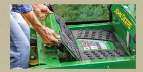
**Head-to-toe comfort.** Adjustable, three-position foot platform. Find the perfect angle and fit for your body whether you have long or short legs. Standard floor mats also enhance comfort by reducing any vibration to your feet. Done mowing? The platform detaches for easy clean-out of mower deck.
