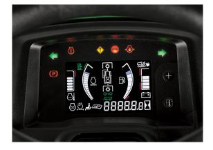
**The dashboard approach** — Electronic Fuel Gauge. Engine Temperature Gauge. Tachometer with Best Cut Target Zone. An Electric Power Take-Off (PTO) engagement indicator. All at a glance and within easy reach.
