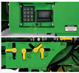
Exclusive Load Command™ system (above left) dramatically cuts loading time on the R4045 Sprayer only. Load the 4,500 L tank as fast as three minutes. System automatically disengages when your sprayer tank is full. Plus, there's reduced risk of any product exposure.
