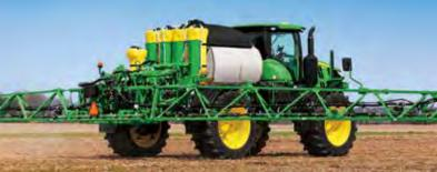
**Direct Injection system** increases your flexibility by changing rates and products on the fly without stopping to mix. The integrated system injects products directly into the system at the boom. The results: quicker changeovers, increased flexibility and lowered risk of using multiple products.
