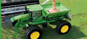
1.5 m (5 ft.) dual bin insert with 1.87 cu. m (66 cu. ft.) capacity on DN456 and 3.00 cu. m (106 cu. ft.) on the DN485.
