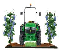
**5GN** Narrow vineyard Engine power: 56, 63, 74 kW (75, 85, 100 hp) Maximum width: 1,785 mm
