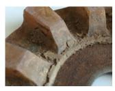
The doffer pad on the right was exposed to a lesser quality product, making it brittle and prone to wear and chunking.
